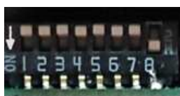
Figure 5: DIP switch positions for default (115200 or flash) and forced (9600) baud rates.
