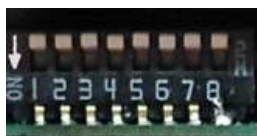
Figure 4: DIP switches in default position (OFF).
